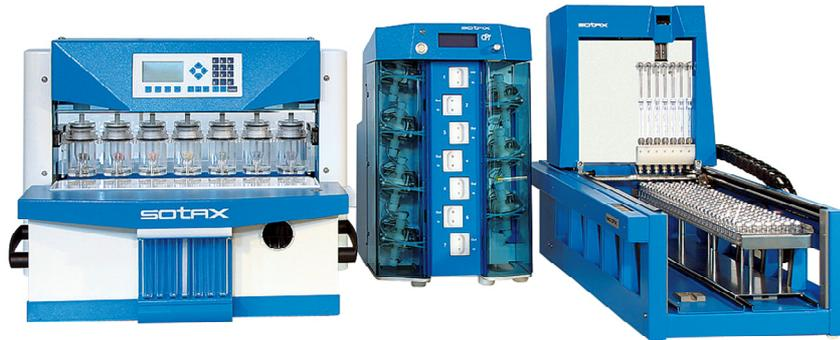
The small volume SOTAX CE 7smart system with MicroVolume Autosampler was developed in 2007 for release rate testing and elution testing of very low dose products such as drug eluting stents, implants and injectables. The microvolume autosampler can take accurate samples as low as 100 ul into capped vials. To increase throughput, two USP IV systems can be run in sequence to one autosampler.
